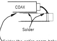
Solder the entire seam between the Coax and the Antenna.
